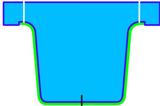
1) gelcoat the male mould and wrap it in a glass material with integral infusion medium like Saercore, or Rovicore
